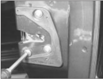
14.4A Unscrew the lock mounting bolts . . .
