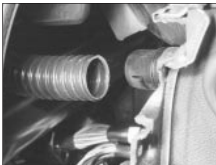
33.22 Disconnecting the fresh air hoses
