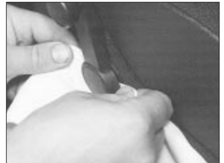
11.7A Using a clean cloth to release the spring clip from the window regulator handle
