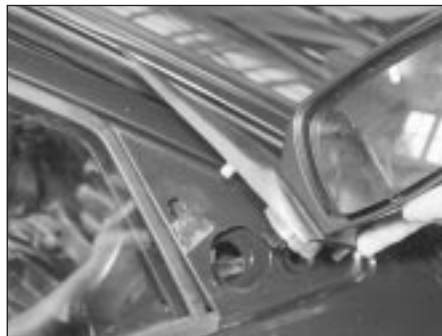
16.5B . . . and withdraw the mirror
