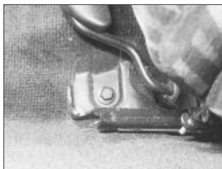
27.5 Front seat front mounting bolt
