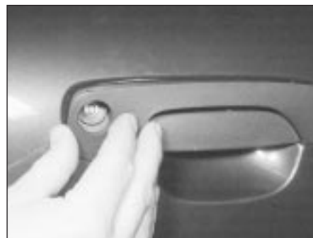
14.3B . . . followed by the exterior handle bezel
