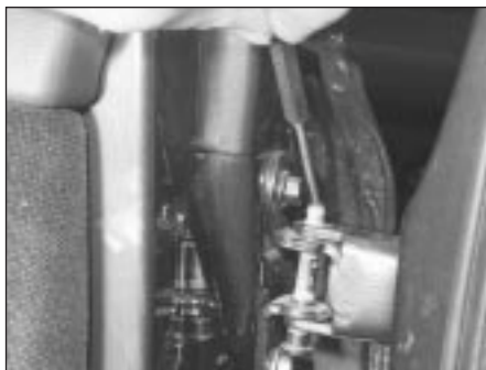
15.5A . . . then drive out the hinge pins . . .
