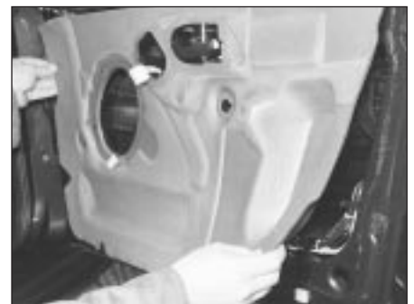
11.12 Removing the foam insulation
