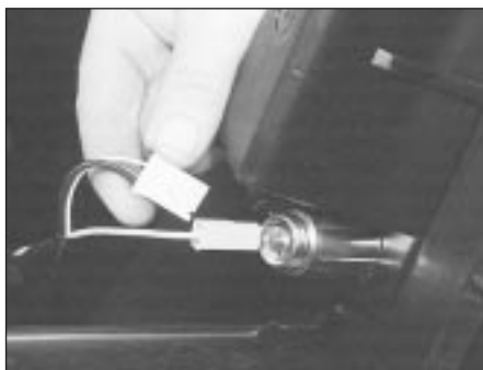
30.8 Disconnecting the cigar lighter wiring
