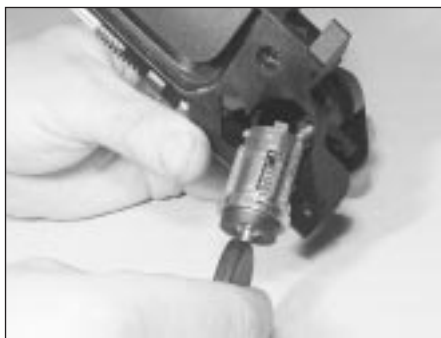
14.25 . . . and pull out the lock barrel
