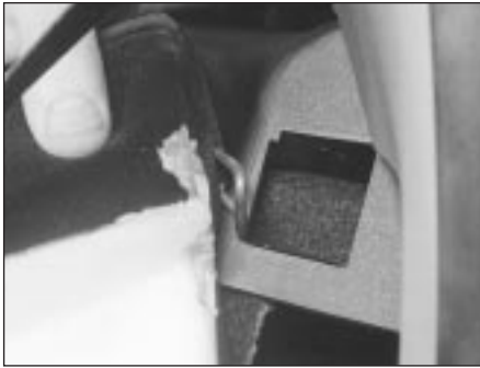
29.15B . . . and release the upper hook
