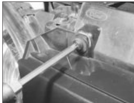
7.2 Removing a radiator grille mounting screw
