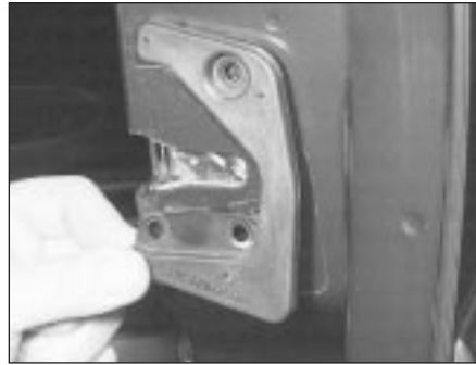
14.4B . . . and remove the plate
