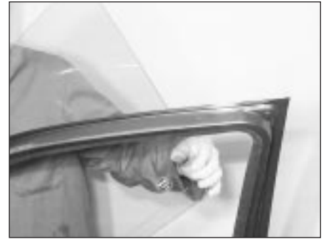
12.15 Lifting the glass from the front door
