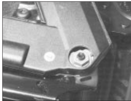
28.4B Front seat stalk mounting nut
