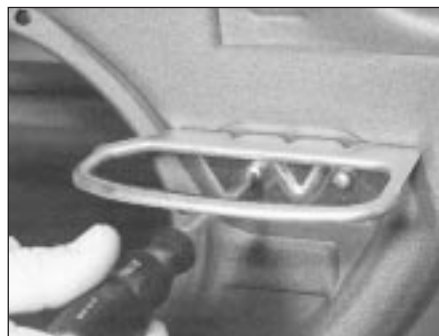
11.11 Removing the door pull bracket from a rear door
