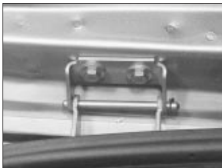
20.24 Tailgate hinge and bolts - Estate models
