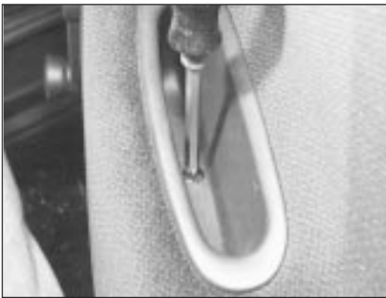
11.6A Remove the screw . . .
