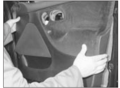
11.8D ... then lift off the trim panel
