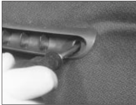
11.4B . . . then remove the screws and withdraw the door pull handle
