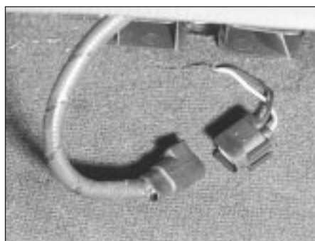
27.4 Disconnecting an electric seat multi-plug
