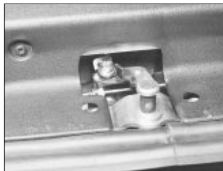
22.24 Lock striker assembly - Estate models
