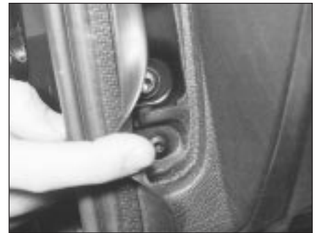
33.18B . . . and pull away the weatherstrip to reveal the facia mounting bolts
