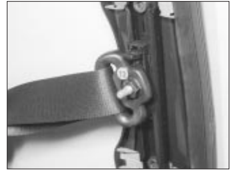
28.3B Front seat belt shackle and mounting nut
