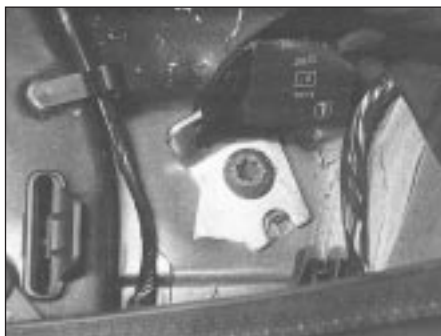
28.8 Rear seat belt lower anchorage
