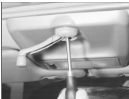
31.3 Removing the sunroof handle securing screw
