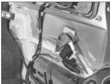
22.6 Tailgate lock barrel and bracket
