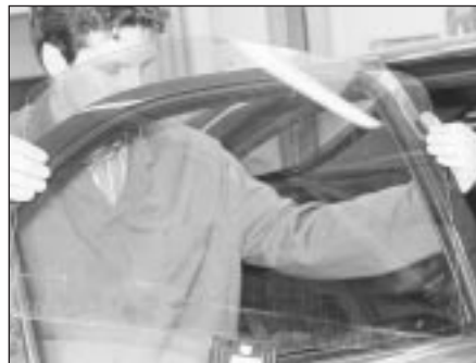
12.26 Lifting the glass from the rear door
