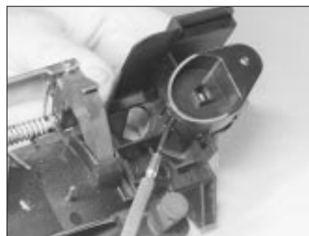
14.24 Prise out the barrel retaining tab . . .
