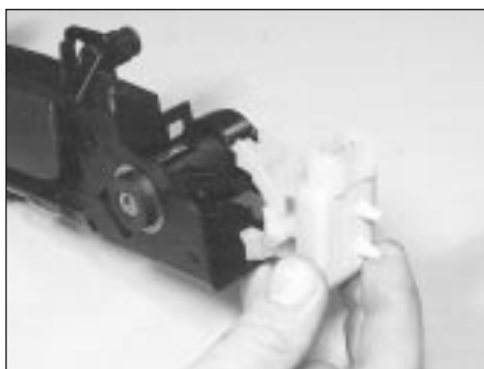
14.11 Removing the central locking "Set-reset" sensor
