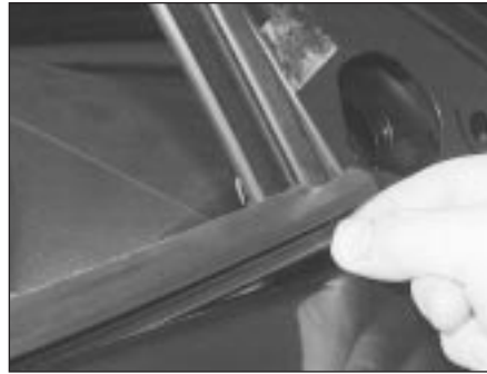
12.13 Removing the weatherstrip from the outside of the door
