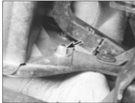
6.5A Front bumper mounting bolt (arrowed)
