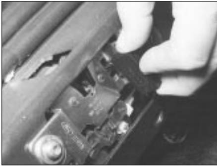
22.14 Removing the door-ajar sensor from the lock
