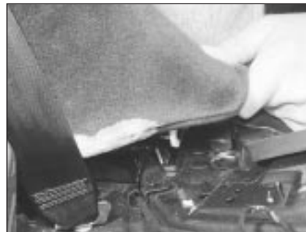
29.15A Pull up the rear seat bolster . . .
