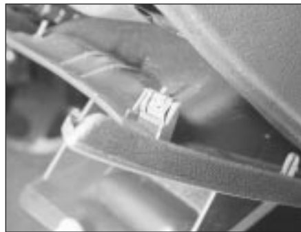
29.23C . . . and withdraw the lower fascia panel
