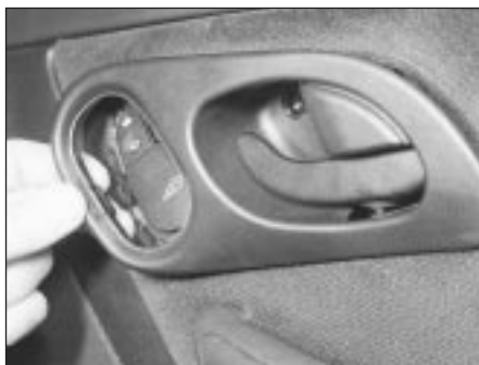
11.2C . . . and withdraw the bezel from the inner door handle
