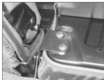
27.10 Rear seat backrest mounting bolts
