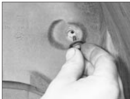
34.3 Removing a wheel arch liner retaining screw
