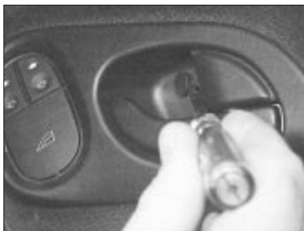
11.2A Prise out the plastic cover . . .
