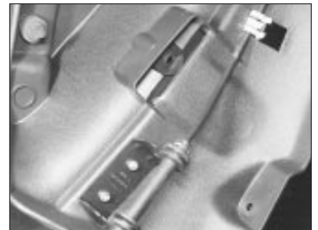
28.6A Detach the rear seat release cable
