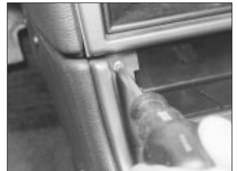
30.6B . . . and unscrew the mounting screws at the front top . . .
