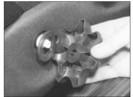
28.5A Remove the recline adjustment knob ...
