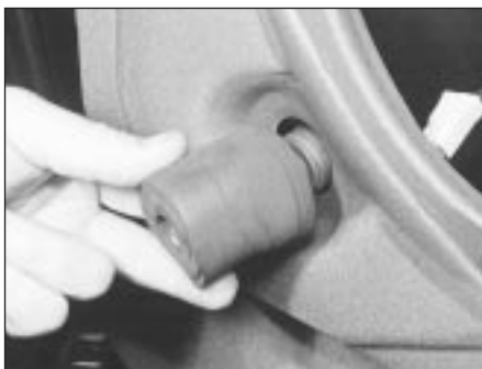
11.10 Removing the foam spacer
