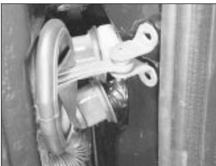
15.2B Front door check strap removed
