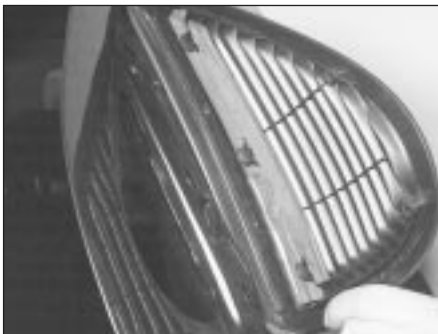
12.21B . . . and remove the air vent grilles from the rear door
