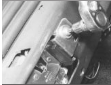
22.15 Removing a lock mounting screw
