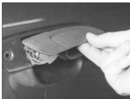
14.16 Removing the rear door exterior handle
