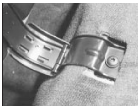
27.6 Rear seat cushion hinge bolt
