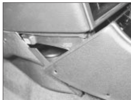
30.7A Withdrawing the front of the console from the fascia
