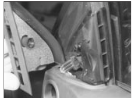
11.5B . . . then withdraw the quarter bezel
