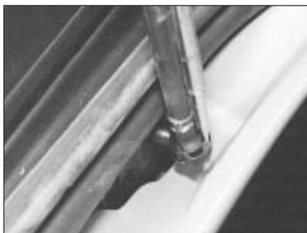
21.3 Prising the spring clip from the lower end of the strut
