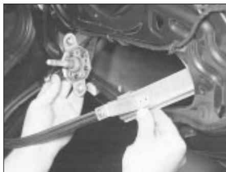
13.6C Removing the window regulator mechanism from the rear door
