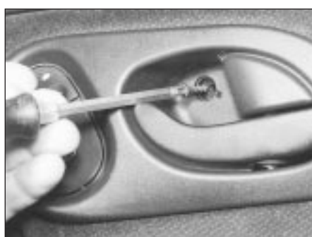
11.2B . . . remove the screw . . .
