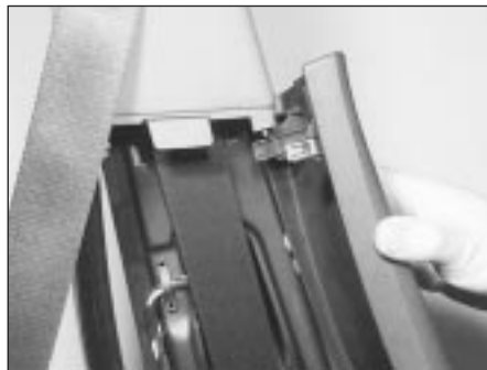
29.11 Separating the "B" pillar lower and upper trim
