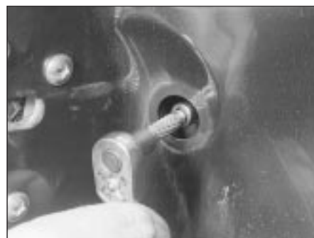
14.14B . . . and unscrew the handle mounting nuts
